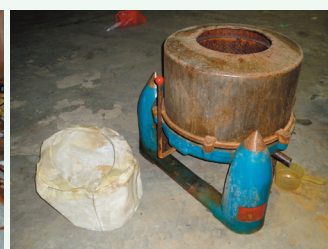
Fig. 6: Centrifuge to spin dry the intermediate product
